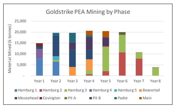
Figure 16-4: Mining production by phase
