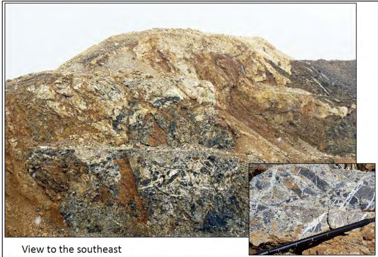
A large collapse breccia body occupies the southeast portion of the A pit. Limestone and dolomite clasts in a matrix of sand and calcite cement, giving way to nearly all calcite near the top of the body. Reddish-brown, elongate zones are lamprophyre dikes, which crosscut the breccia, but can also be found as clasts in it. Inset: detail of breccia with angular limestone clasts in a sandy, calcite cemented matrix.
