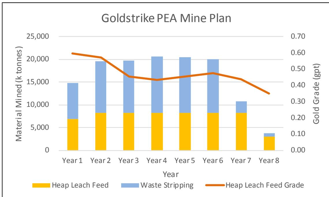
Figure 16-5: Mining production showing waste stripping and head grade
